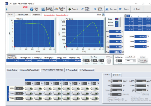
Fig. 15. Control panel for photovoltaic simulator output characteristics.
